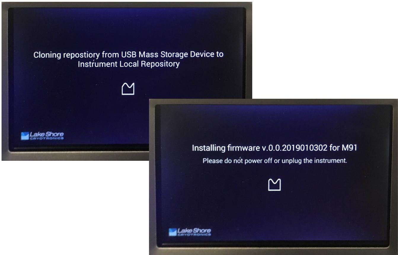
6. When complete, the instrument will return to its home screen and be fully functional again. Remove the USB flash drive, otherwise the operating system will be reinstalled every time the instrument boots up.
