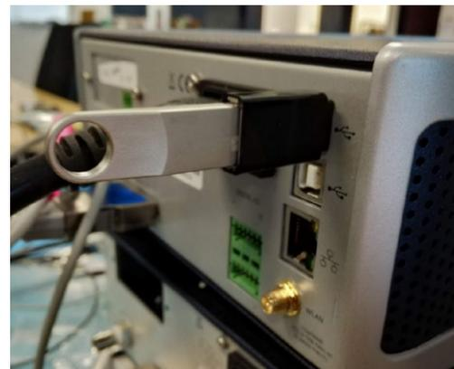
3. Press the power button again until it turns on, or return power to the instrument. The update process will begin automatically. The update process should take 5 to 10 minutes. None of the standard instrument functionality is available during the update.
