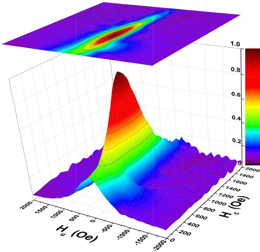
Figures 4 and 5 show the measured FORCs and the FORC diagram, respectively, for sample B.<sup>2</sup> There are 9,045 points in the FORCs and the total measurement time was 1.5 hours. Note that the moment at maximum field is approximately 0.8 memu, which is approximately 25 times lower than sample A, thus illustrating the speed of the PMC VSM, even for relatively low moment samples.
