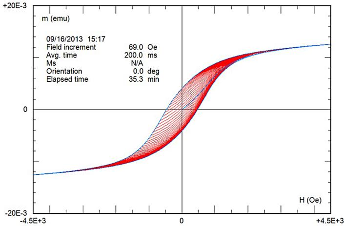
Figure 1 shows the initial magnetization curve and major hysteresis  $M(H)$  loop (blue) and a series of FORCs (red) for sample A. There are 5,940 points in the FORCs, and the total measurement time was only 35.3 minutes, which illustrates the speed of the PMC VSM.
