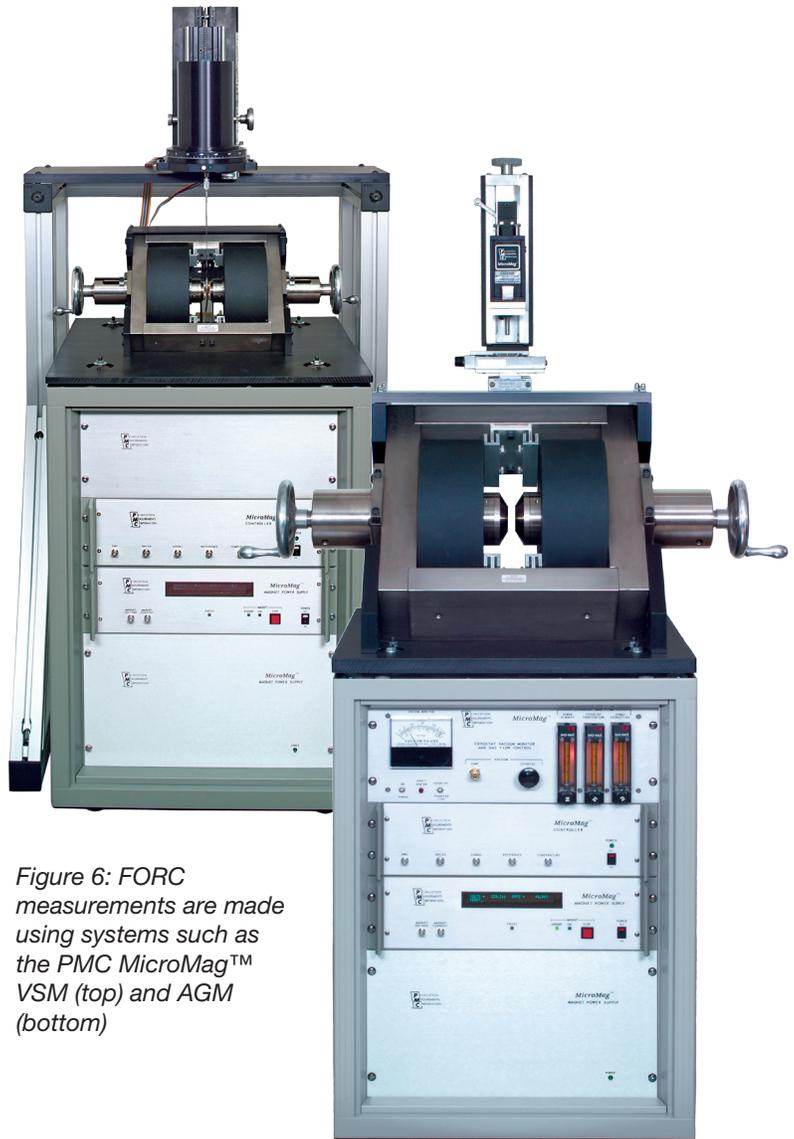
*Figure 6: FORC measurements are made using systems such as the PMC MicroMag™ VSM (top) and AGM (bottom)*
