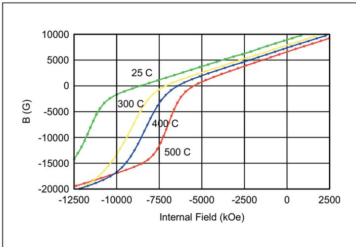
Figure 5  $B(H,T)$  curves for SmCo magnet material.
