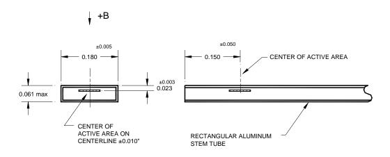
Note that the "active area" of the probe is closer to one side. This side should be nearest to the mass standard during measurement. An easy method of insuring that this is the case is to position the Lake Shore logo on the probe handle towards the weight.
