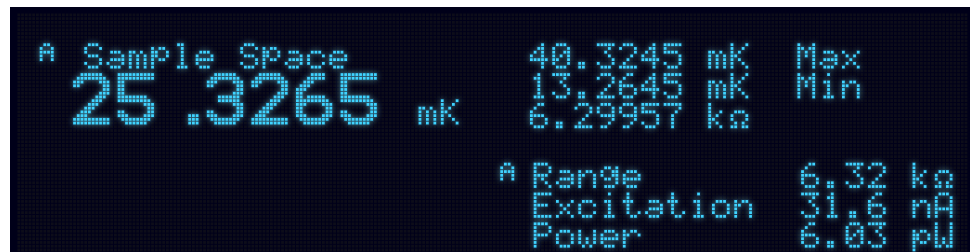
FIGURE 4-6 Control input display mode
