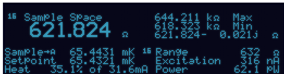
FIGURE 4-9 Control/scan information display quadrant configured to display sample heater A
