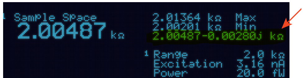
FIGURE 2-4 Display showing impedance measurement
