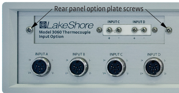
FIGURE 7-4 Correctly orient the option card (thermocouple input option card shown)
