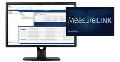
MeasureLINK software enables a wide range of capabilities including charting and logging, system monitoring with a cryostat-specific process view, and controlling Lake Shore equipment as well as third-party instrumentation. No programming required – drag-and-drop to create temperature sweeps, access measurements, and see real-time internal cryostat temperatures in process view.
