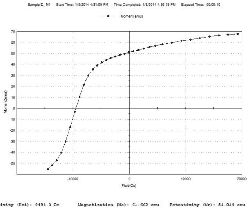
Figure 1—Demagnetizing process for a permanent magnet material sample, as measured with the model 7410 equipped with a guide tube. The notable fact is the ability to measure large moment samples, 50 emu in our case, a typical situation encountered in industry. Without the guide tube, one has to cut the sample down to very small dimensions ( $2 \times 2 \times 2$  mm) in order to reduce the magnetic moment and, consequently, the pull force.
