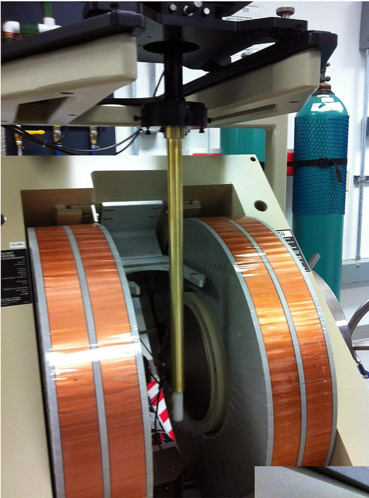
*Figure 4—For easy sample replacement, the head slides forward. This is another advantage of attaching the guide tube to the head drive.*
