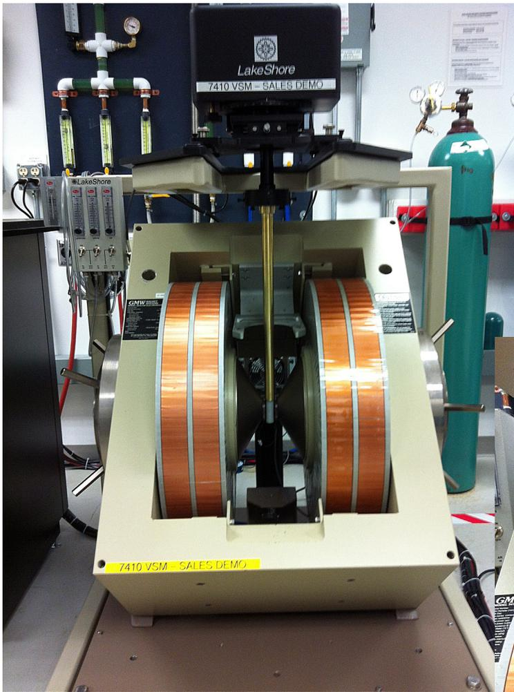
Figure 2—Complete view of the Model 7410 with the guide tube installed. Retrofitting an existing VSM to use this fixture is a simple, 5 minute, straightforward process. Attaching the option directly to the head drive enables us to avoid any increase in measurement noise.
